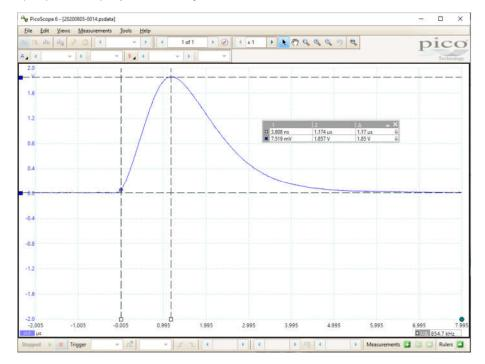
Corresponding unfiltered detector signal (measured with CP10B fast pre-amplifier)
