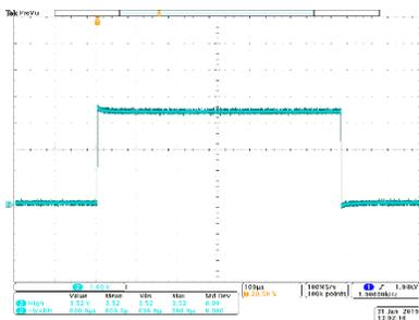
Typical Output Waveform, 3500 V Output, at V-Mon
