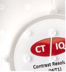
Leeds Test Objects' CTIQ Image quality phantom is designed for use with CT (Computed Tomography) units. CTIQ comprises a PMMA cylinder (160mm diameter, density  $1.20 \pm 0.01$  g/cm<sup>3</sup>) with recesses to house test inserts.
